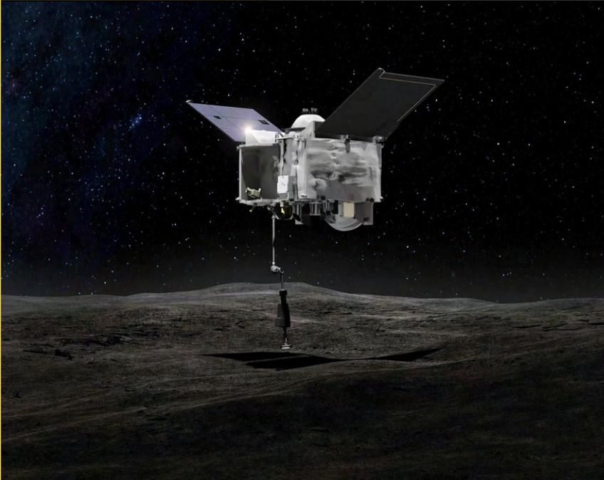
*This artist's concept shows the OSIRIS-REx spacecraft contacting the asteroid Bennu with its Touch-And-Go Sample Arm Mechanism, or TAGSAM. Image by NASA Goddard Space Flight Center*
