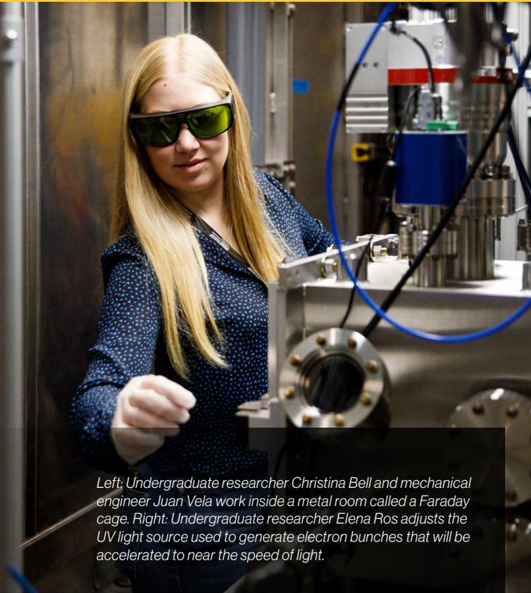
*Left: Undergraduate researcher Christina Bell and mechanical engineer Juan Vela work inside a metal room called a Faraday cage. Right: Undergraduate researcher Elena Ros adjusts the UV light source used to generate electron bunches that will be accelerated to near the speed of light.*
